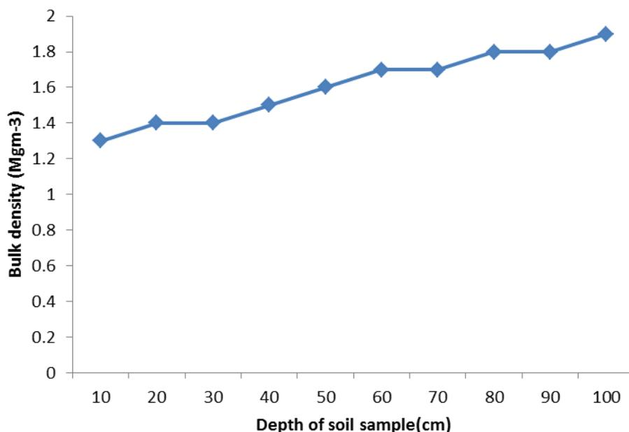
**Figure 2.** Bulk Density increases with Soil Depth.
